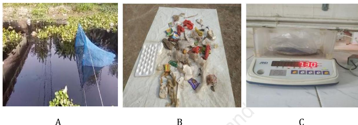
Fig. 2 Sampler installed (A), exposed to air (B), and weighed (C) individually procedure for plastic debris.
